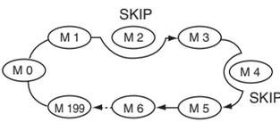
Repeatedly scans memory channels, except those set as skip channels. Used for often-called channels and for bypassing normally busy channels such as **repeater** frequencies.
