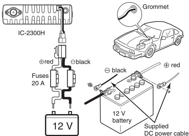
**NOTE:** Use terminals for the cable connections.
