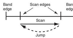
Repeatedly scans between two programmed frequencies. Used to checking for frequencies within a specified range, such as **repeater** output frequencies, and so on. 3 pairs of **scan edges** are programmable.
