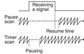
11 pause options and 7 timer options are selectable. When receiving a signal, the pause scan pauses until the signal disappears; timer scan pauses for the specified period of time.
