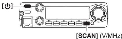
➔ While holding down [V/MHz], hold down [POWER] for 1 second to reset the CPU.
