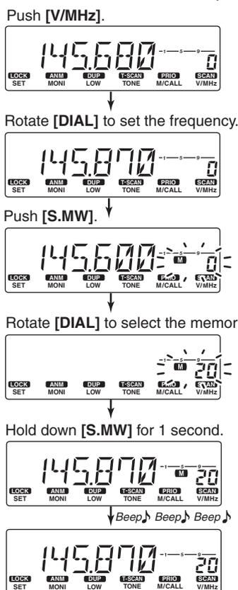
[i.e.]: Programming 145.870 MHz into the memory channel 20, using the microphone.
