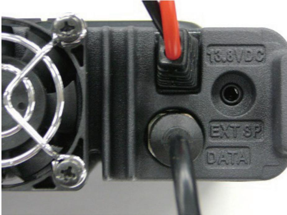
Connect the opposite end of the data cable to the USB port or the COM port of the PC. (Photo shows the SCU-20)
