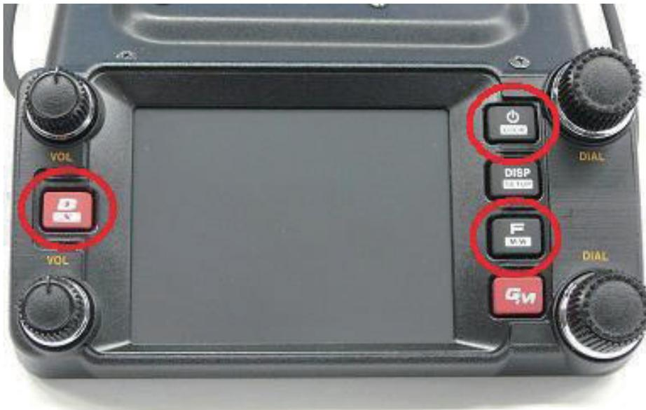
After “PUSH D KEY” appears on the screen, press the [D/X] key.
