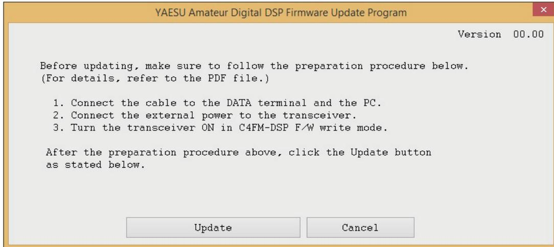
The procedures required to prepare the transceiver to receive the firmware update are listed, carry out the respective tasks as follows:
