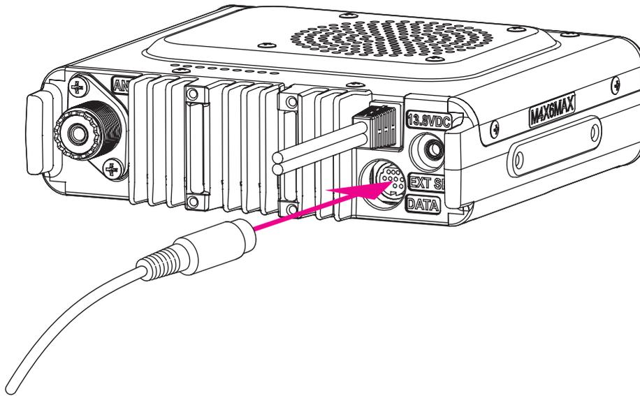
Connect the opposite end of the data cable to the USB port or the COM port of the PC. (Figure shows the SCU-20)
