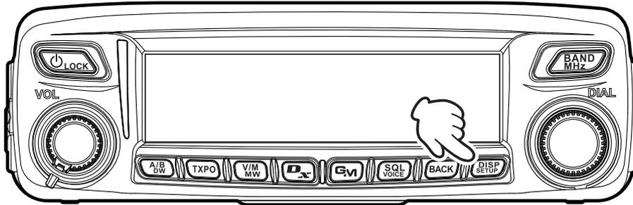
3. Rotate the DIAL to select [13 RST/CLONE], and then press
